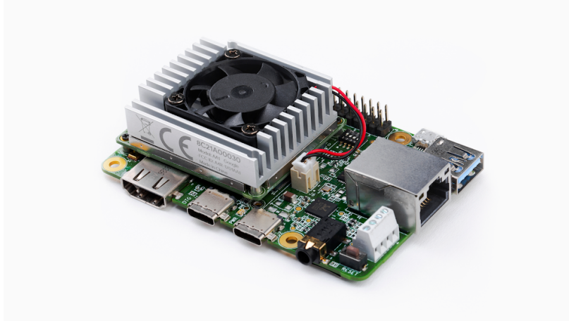
Figure 31: Edge TPU - Dev Board https://coral.ai/products/dev-board/
